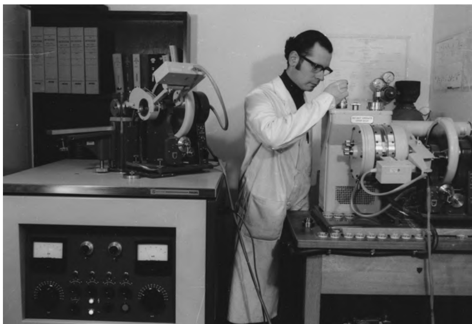
State of the art X-Ray equipment, 1960's. The late Dr Tony Weir is inserting a pressed powder pellet for XRF analysis. XRD machine is on the left. One generator served both machines.
